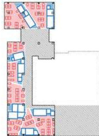
⑤ Automated "test fit" generates amenity rooms from space matrix and desk layout.
